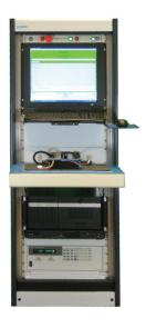
The ASE SSL 3.0 Test System can be used for testing of single or multi-channel LED drivers, either constant current (up to 20A) or constant voltage (up to 500Vdc). The system is easily configured to meet end user requirements in order to optimize hardware and minimize test cycle time.
